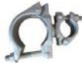
FF-0908T AMERICAN TYPE SWIVEL COUPLER 89mmX48.3mm 2.95 KGS
