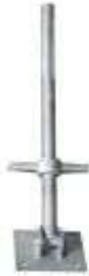
EK-SJ001 旋转调节底座 Swivel Adjustable Screw Jack Base 600 914mm 35/38mm 150X150X8mm
